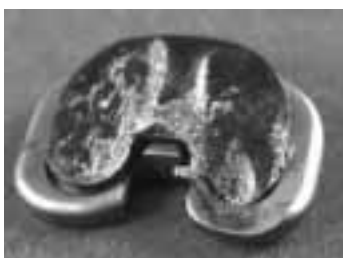
Figure 6: A failed Poly-2 tibial insert retrieved 5 years after implantation.
