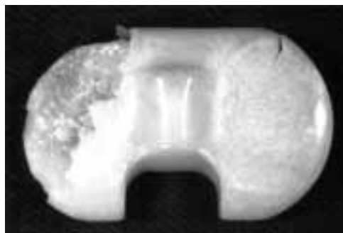
Figure 4: A Group 2 plateau implanted after 7.6 years of shelf storage and retrieved 3.8 years after implantation. Gross delamination and pitting, characteristics of fatigue failure, are observed.
