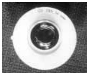
Figure 7: A failed Hylamer acetabular cup insert retrieved 3 years after implantation.
