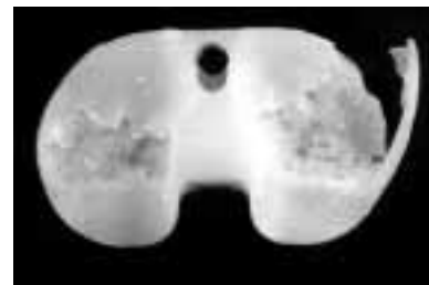
Figure 8: A heat pressed tibial component retrieved 6 years after implantation.
