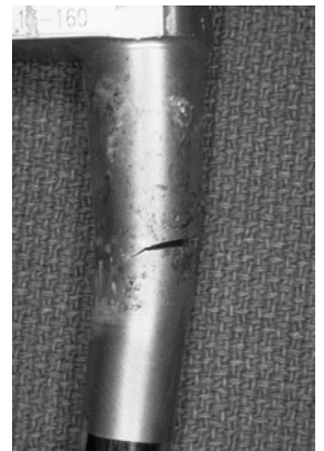
A close-up A-P view of the fracture site.
