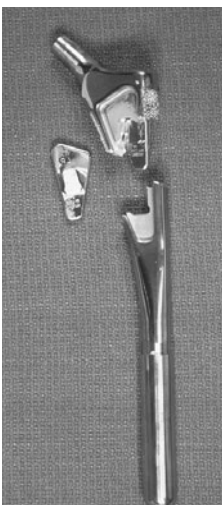
A-P view showing a failed device.
