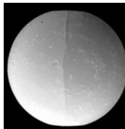
Classic Diametral Tension Fracture
