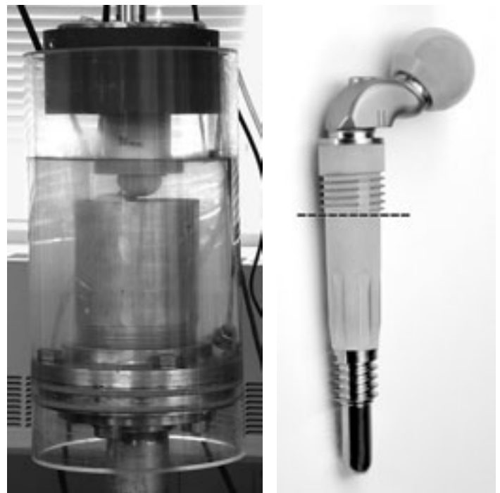
Figure 1: Test Assembly and Potting Level (-----) .
